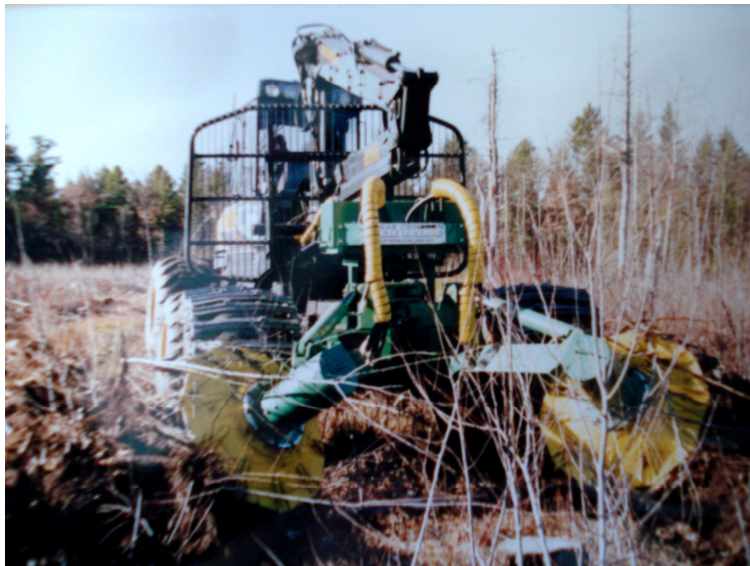
Figure 6.2 Disc Trenching equipment used to prepare sites for planting.
